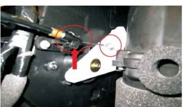
13 取掉空调拉线
