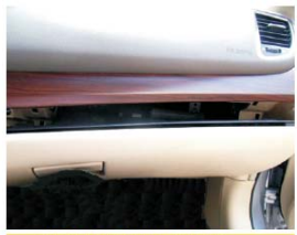
60 将储物箱安装回原卡位，固定6颗螺丝
