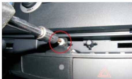
17 拧下应急灯面板的螺钉
