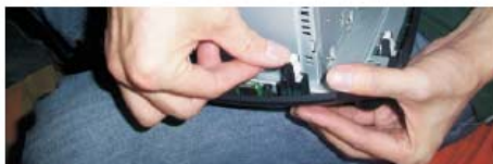
10 把中控大盖左右两侧一颗螺丝拆掉
