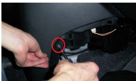
10 把中控大盖左右两侧一颗螺丝拆掉
